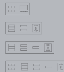
Horizontal multi-gang installation
