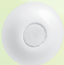
0 488 04 PIR ceiling mounted Lighting Management Sensors 360° infrared detection, ø8m range Additional 2A contact for HVAC control based on presence data Surface mounting on ceiling using accessory
