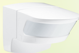
0 488 10 270° outdoor sensor IP 55 Detection field 180m 2 - For building entrances, car parks PIR - Max range 15m Front detection 10m Lateral detection 30m (2x15) Dual side detection specially adapted for wide areas (example: entrance hall)
