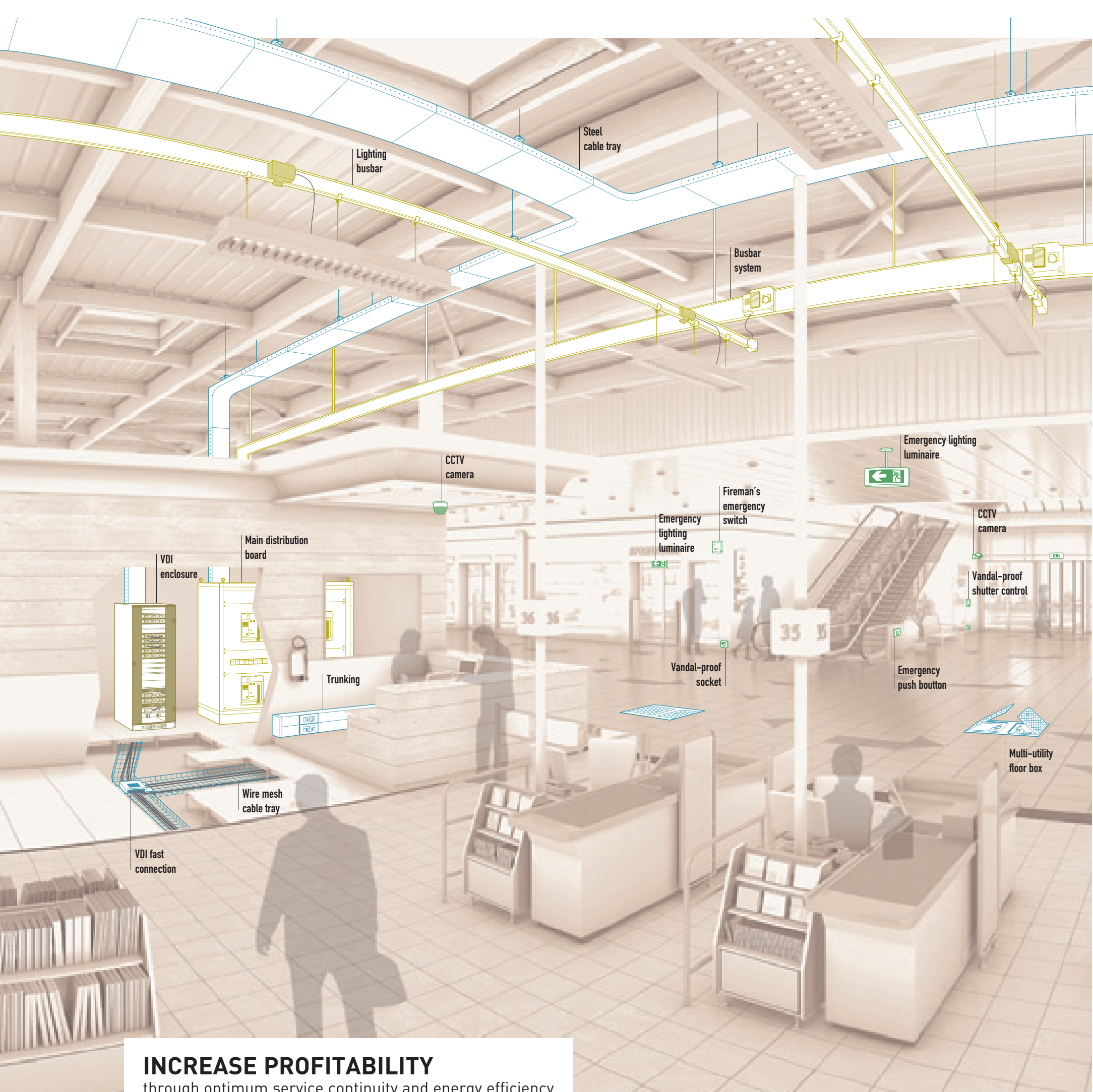
Cablofil® wire mesh cable tray: safe, quick and easy fit
